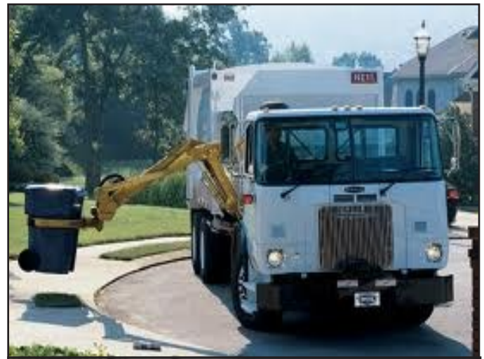
Automated Collection Vehicle with robotic arm
